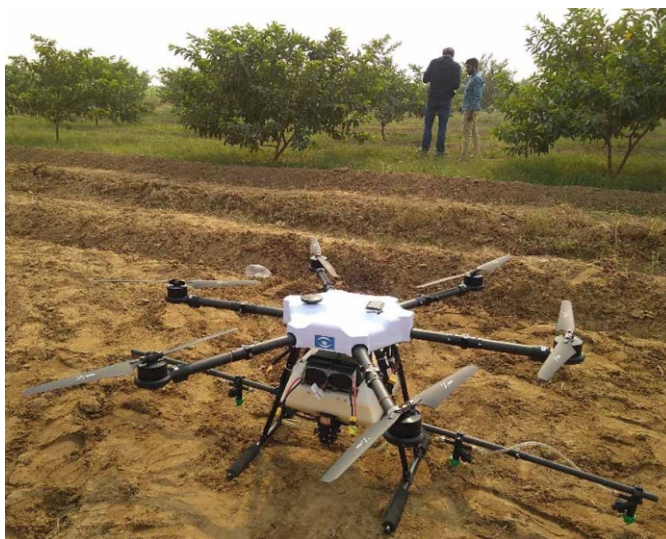
Fig. 1: A view of the UAV used for spraying in orchards.
